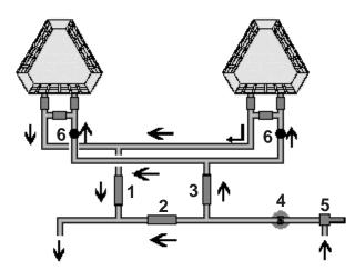
For some larger pools, it may be necessary to install two units in parallel. In this case, double the distances recommanded in the table 1 of the page 5. Never place two MP models coil against coil, fan against fan or coil against fan.
